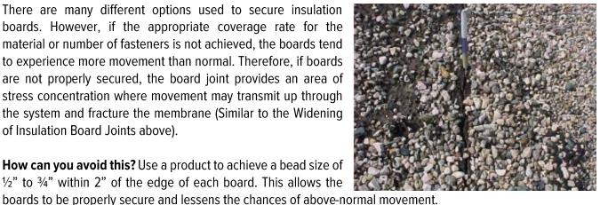
Regardless of the method of attachment used, be sure to read the specification pages to ensure the proper coverage rates or fasteners are used to secure the boards.
